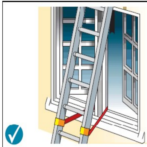
Ladder tied at the top stiles (correct for working on, but not for access)
